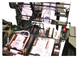
Two-Up Feeder Attachment (optional) One of the many accessories available for the Kluge EHD is the two-up feeding attachment. Adding twoup feeding capability to your press enables you to run two jobs simultaneously or the same job at double the productivity.
