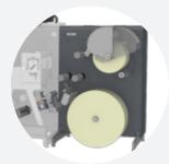
**GM SmartTurret** - NEW fully servo controlled automatic turret rewinder. Provides efficient production without stopping when changing rolls.
